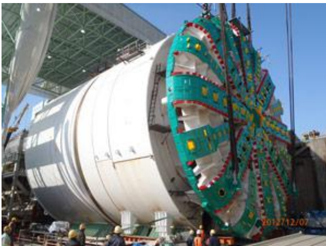
Tunnel boring machine used on Alaskan Way Viaduct Source: Washington State Department of Transportation
